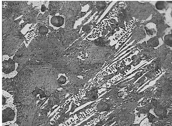
Fig. 1. Carbides in DCIs (500 \times ).
