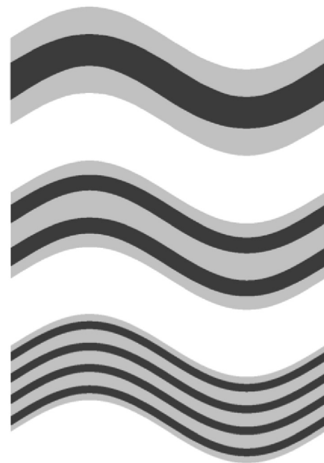
Fig. 2. Unit cells of the lamellar material comprised of sinusoidal architectures (amplitude-to-wavelength ratio of 0.1) with a fixed volume fraction of the hard phase layers of 0.40 (dark region), which are subdivided into progressively thinner plies.
