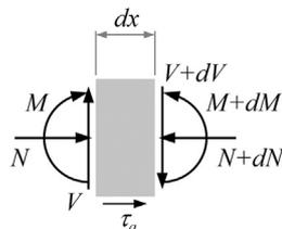
Fig. 2. Forces acting on an infinitesimal element of an AB3PB specimen upper adherend.
