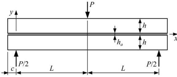
Fig. 1. The adhesively bonded three-point bending (AB3PB) specimen.
