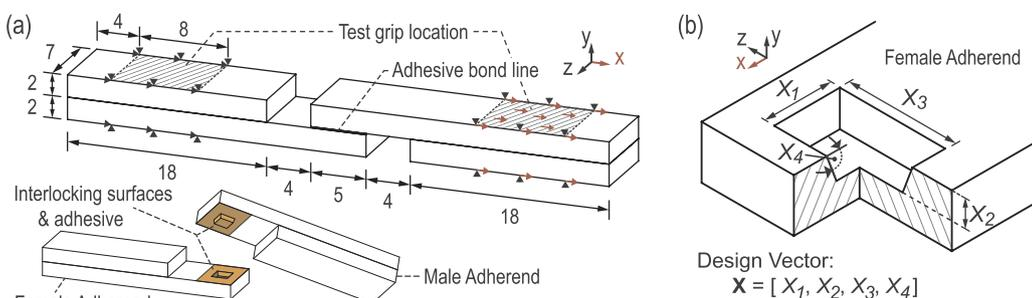
Fig. 1. Miniature SLJ (a) geometry and boundary conditions, with dimensions in millimetres and (b) truncated, square pyramid interlocking profile geometry and corresponding geometric factors.
