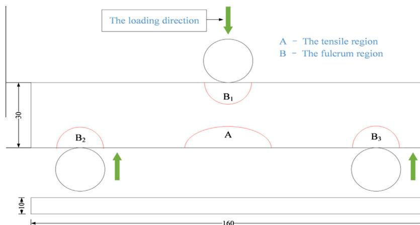
Fig. 1. The shape and dimension of specimens.
