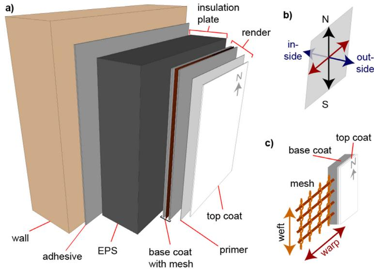
**Fig. 1.** (a) Design of External Thermal Insulation Composite Systems (ETICS) as used in this study, consisting (from wall to outside) of an adhesive layer (2 mm), an insulation plate (expanded polystyrene EPS, 80 mm), a base coat (4 mm) with reinforcement mesh and a top coat (layer thickness 1.5 mm). (b) Sample orientations used in this study: North direction toward the roof and inside toward the house wall. (c) Close up of the render showing the reinforcement mesh string orientation.
