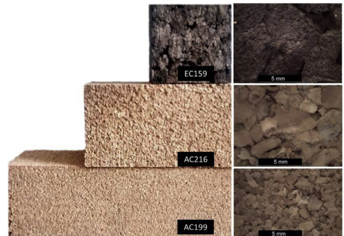
Fig. 1. Cork agglomerates studied: From top to bottom (EC159: expanded, large grain black cork; AC216: medium grain, white agglomerate; AC199: small grain, white agglomerate).
