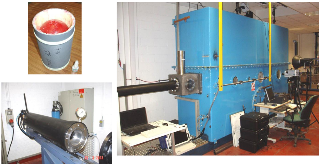
Fig. 1. Ghent University bird strike test set-up: a sabot with a gelatine bird (top left), the pressure vessel (bottom left) and the stripper and test chamber (right).
