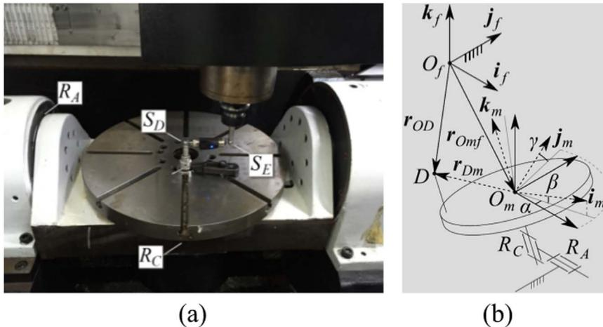
Fig. 1. The devices of ball bar testing.
