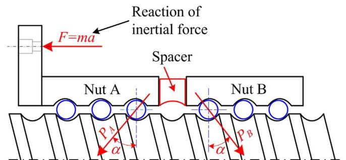
Fig. 3. Cross-section view of a gasket-type double-nut ball screw joints.
