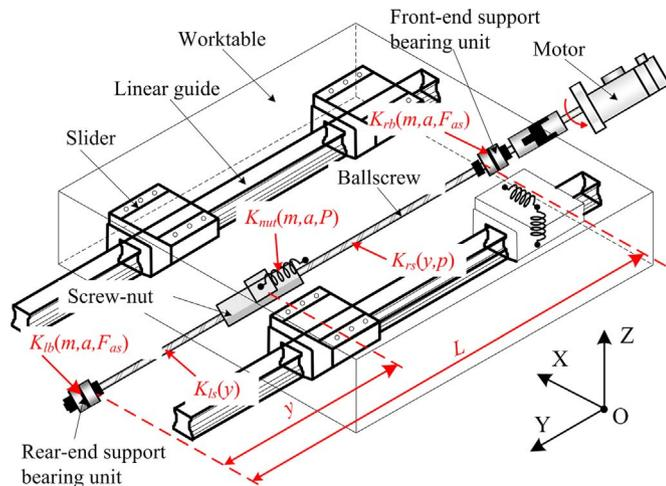
Fig. 1. The structure of a ball screw feed system.
