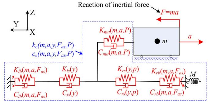
Fig. 2. Equivalent dynamic model of the ball screw feed system with high acceleration.
