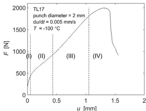
Fig. 2. Force-deflection curve for a tensile SP test of a Grade 91 stainless steel at  $-100$  °C [12].
