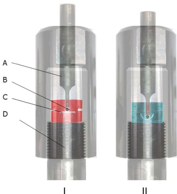
Fig. 1. Typical SP test setup: I. Modified SP test setup for tube specimen; II. A) puncher, B) puncher ball, C) specimen, D) clamping thread.
