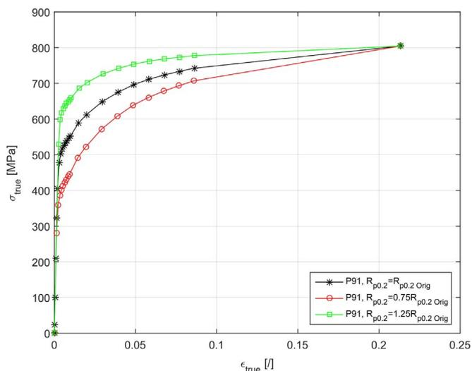
Fig. 3. P91 true stress-strain curves.
