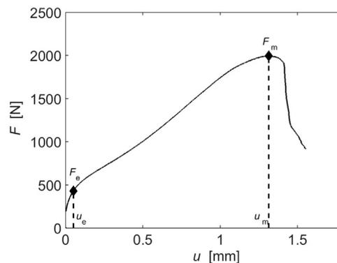
Fig. 4. Locations of the parameters  $F_m$ ,  $u_m$ ,  $F_e$  and  $u_e$  from the force-displacement curve.
