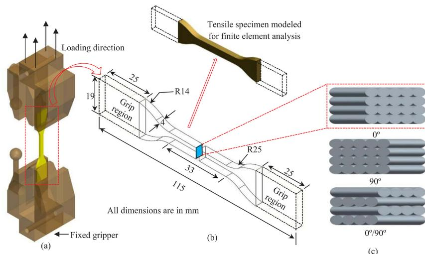
Fig. 1. (a) Schematic of gripper arrangement, (b) tensile specimen as per ASTM D638 standard, (c) schematic illustration of different raster angles.
