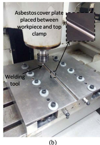
Fig. 1. (a) Fixture model showing detailed parts of the proposed fixture, and (b) Experimental set-up showing the developed fixture used for welding.
