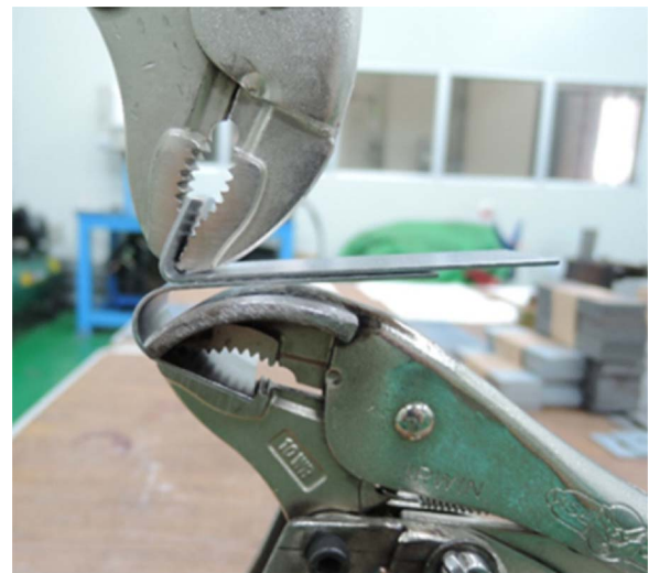
Fig. 1. Peeling test setup.
