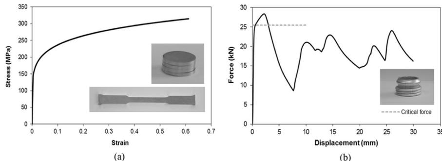
**Fig. 2.** Mechanical characterization of the AA6063T6 tube material. (a) Stress-strain curve obtained from tensile and stack compression tests performed in specimens cut out from the supplied tubes. (b) Force-displacement evolution and critical instability force for the axial compression of the supplied tubes between flat dies.
