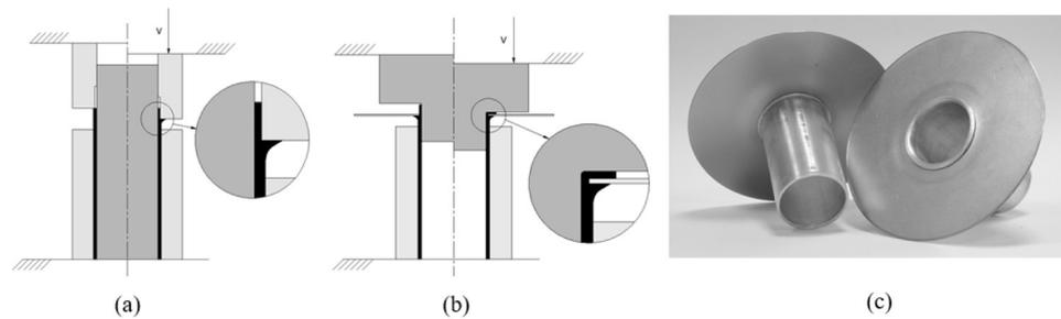
**Fig. 1.** Sheet-bulk forming of thin-walled tubes for joining applications. (a) Schematic representation of material pile-up and localized thickening produced by partial compression of the wall thickness along the longitudinal direction. (b) Schematic representation of the procedure for flaring out (and locking) the upper tube end inserted in the sheet hole. (c) Hollow flanged components produced by the new proposed joining process.
