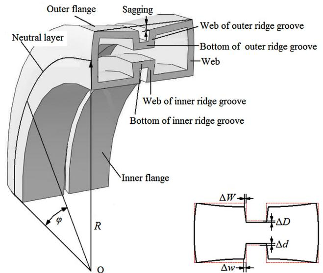
Fig. 1. Schematic illustration of cross sectional deformation of double-ridged waveguide tube in rotary draw bending.
