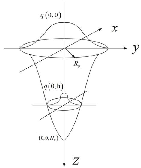
Fig. 1. Laser heat source model (Wu et al., 2004).
