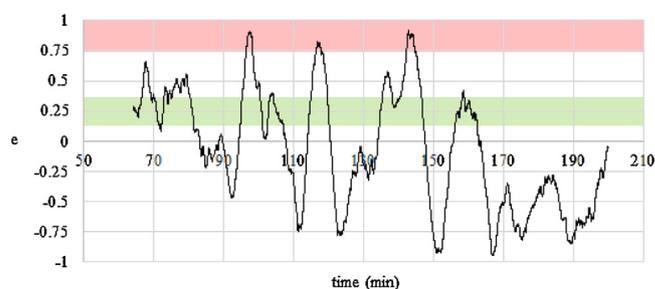
Fig. 1. Fracture growth exponent plot for stage 9 of Eagle Ford shale. Reprinted with permission from Hydraulic Fracturing Journal.
