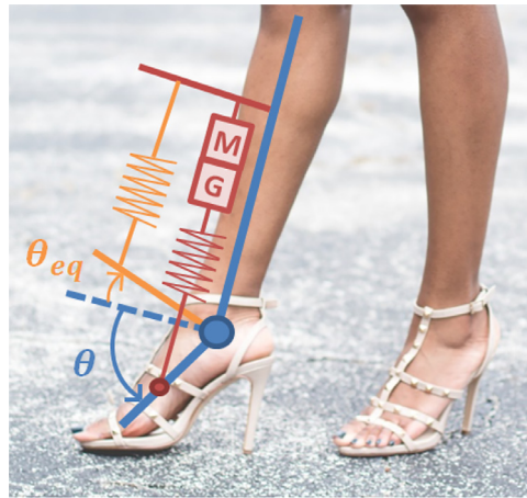
Fig. 1. Schematic of the actuator with angle definitions. The actuator consists of a Series Elastic Actuator (red) and a unidirectional parallel spring (orange), which is engaged when \theta \geq \theta_{eq} . The ankle angle \theta is zero when the foot is perpendicular to the leg (denoted by a dashed line). A plantarflexed ankle, as depicted in the figure, corresponds to a negative value of \theta . Note that, for clarity of the presentation, the elastic elements are drawn as compression springs in the figure, although they are modeled as torsional springs in the work. (For interpretation of the references to color in this figure legend, the reader is referred to the web version of this article.)
