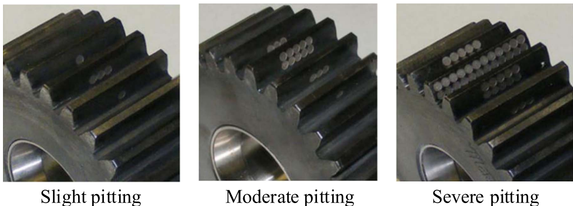
Fig. 2. Planet gears with artificially created pitting damage [11].
