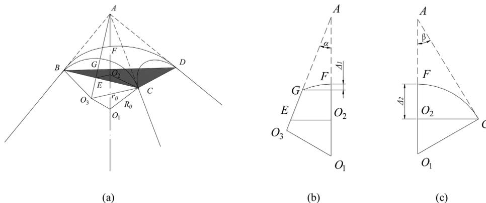
Fig. 2. (a) Spherical capped regular three side pyramidal tip model; (b) Section of the triangle  $\triangle AO_1O_3$ ; (c) Section of the triangle  $\triangle AO_1C$ .
