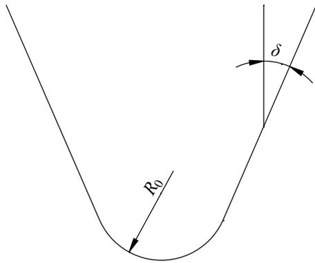
Fig. 1. Spherical capped conical tip model.
