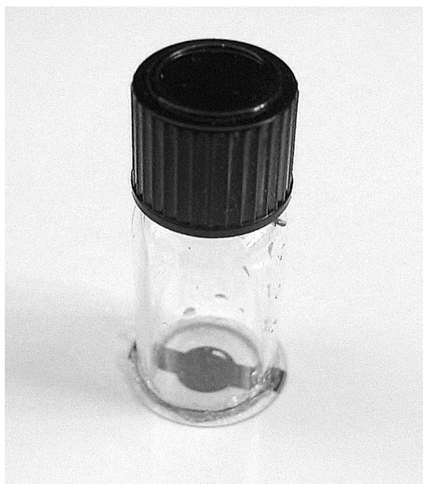
Fig. 1. Test vial with attached crystal.
