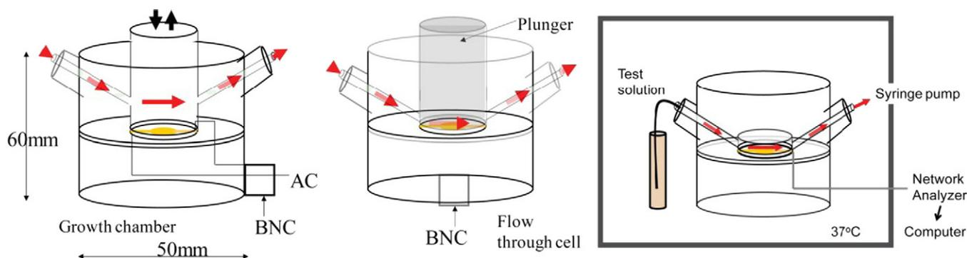
Fig. 1. Left: Static TSM chamber used for neuronal deposition experiments. Middle: Flow TSM chamber used for neuronal studies that require solution flow. Right: Experimental setup enabling temperature control via a hybridization oven set at 37 °C.
