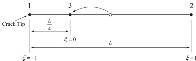
Fig. 1. Nodes on crack tip adjacent side of quarter-point element.
