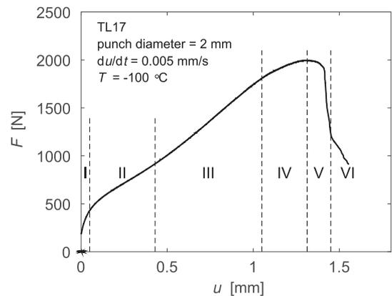
Fig. 2. Typical SP force-deflection curve for a ductile material [17]. The roman numbers indicate the different zones of the curve.
