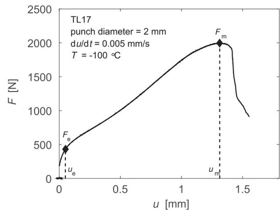
Fig. 3. Characteristic points in the force-deflection curve [17].
