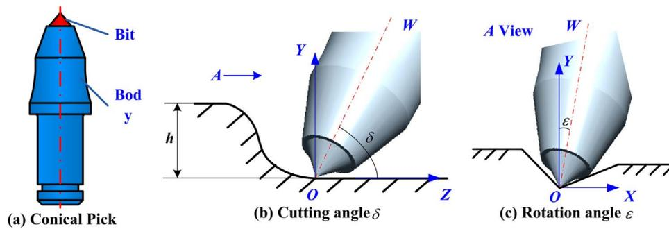
Fig. 1. Conical pick and operating angle.
