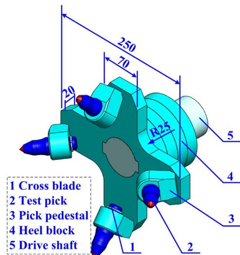
Fig. 2. Structure of the experimental cutting head.
