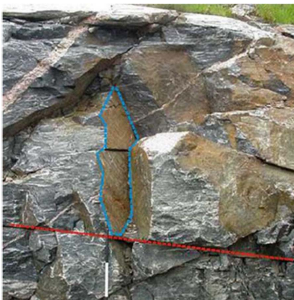
Fig. 1. Two exposure scenarios of discontinuities: facet exposure (cyan polygon) and trace exposure (red line) (after Otoo et al. 30 ). (For interpretation of the references to color in this figure legend, the reader is referred to the web version of this article.)
