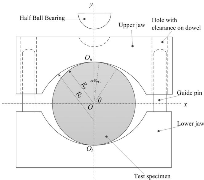
Fig. 1. Suggested apparatus for the execution of the Brazilian test by ISRM.
