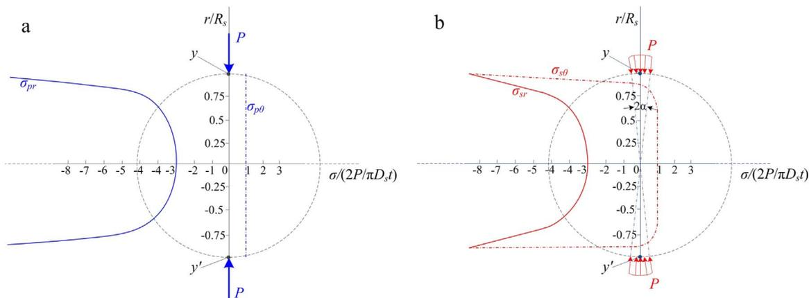
Fig. 2. (a) Principal stress components along the diametric line compressed by a point load; (b) Principal stress components along the diametric line compressed by a strip load. The dashed circle presents the disk specimen. The stress components are normalised by  $2P/\pi D_s t$ , and conventionally, the quantity of the tensile component is positive.
