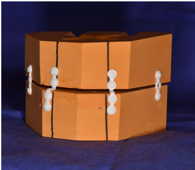
Fig. 1. The experimental set up showing the two cast blocks, reflecting the separated maxillary segments stabilized in the desired position using virtually planned and individual fabricated ZrO 2 mini-plates.
