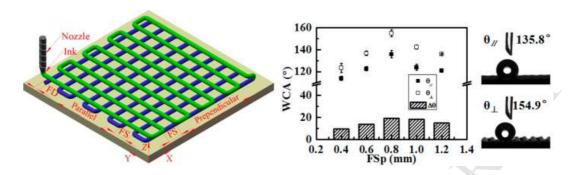
With the guide of computer program for 3D printing, the PDMS porous films can be printed with versatile special surface wettabilities such as anisotropic wettability and superhydrophobicity, and show attracting applications in air-breathable water-proofing, water-repellent floating carrier, and no-loss liquid transfer.
