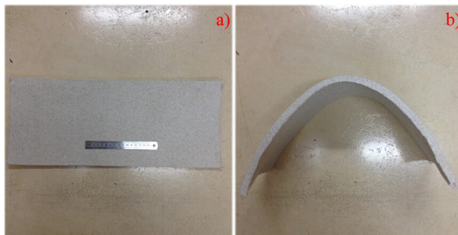
Fig. 1. Photograph of the material. a, before bending. b, after bending.
