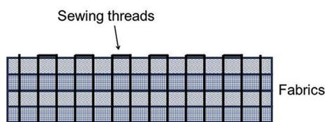
Fig. 1. Schematic of the AS fiber preform employed in the AS/SiO<sub>2</sub> composite in this study.
