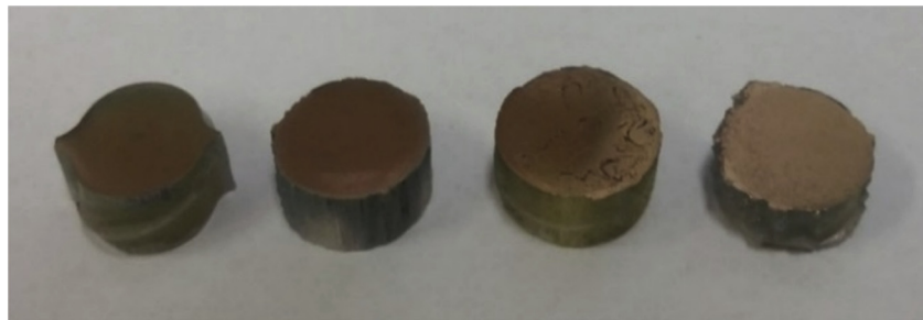
Fig. 1. Representative prepared samples (from left: GFRP-A, B, C, and D).
