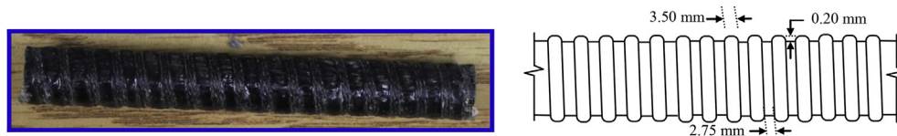
Fig. 1. BFRP bar 12 mm in diameter used in this investigation.
