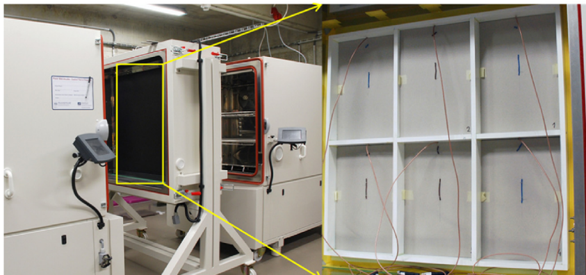
Fig. 1. Double-climatic chamber setup used in condensation experiment.
