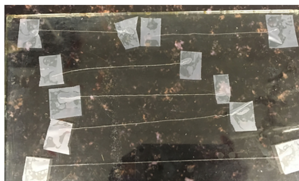
Fig. 1. Drying of wet-spun CNF filaments.
