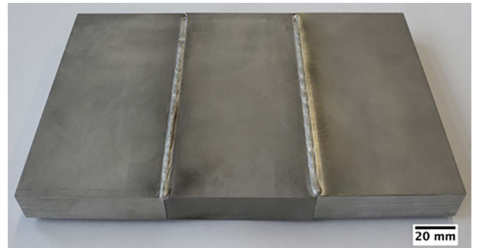
Fig. 1. Welded plates using weld number 2 parameters.
