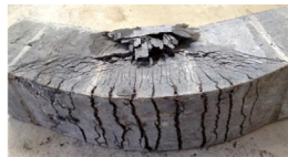
Hybrid steel wire mesh and micro fibre reinforced beam under static flexure
