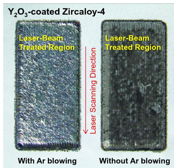
**Fig. 1.** Appearance of the laser-beam-scanned Zircaloy-4 sheet coated with  $Y_2O_3$  (20  $\mu\text{m}$ ) and treated by 180 W laser beam. Left and right regions correspond to laser-beam-treated samples with and without Ar blowing.
