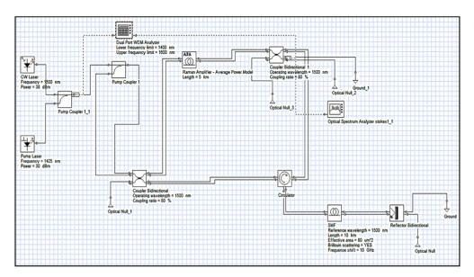
Fig. 1. Simulation Layout of the ring-cavity MBRFL.
