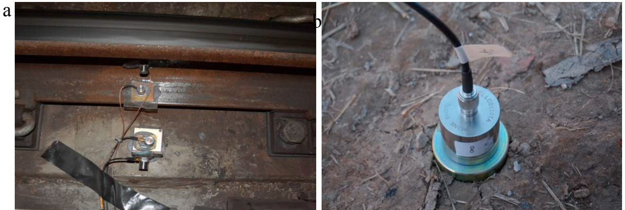
Fig.1.(a) rail acceleration measuring-point arrangement;(b)ground surface acceleration measuring-point arrangement
