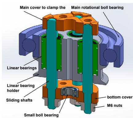
Fig. 2: Section view of rotating hub assembly.
