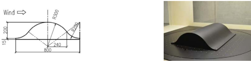
Fig. 1. Scheme of the object which is flown around and a model of this in an aerodynamic tunnel [12], dimensions in [mm].
