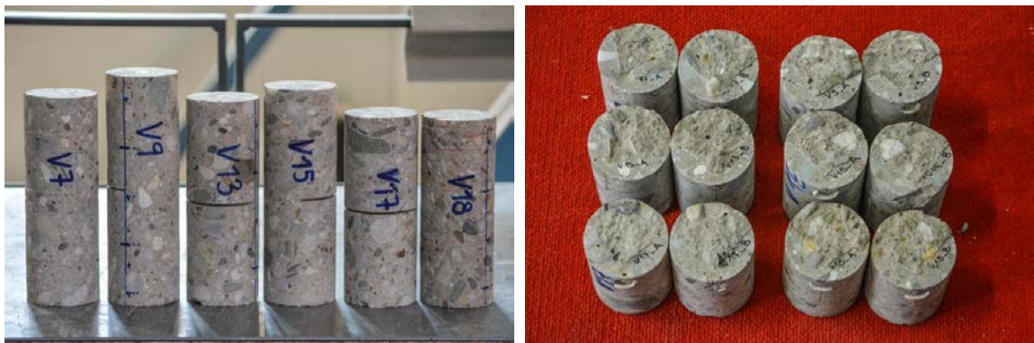
Fig. 1. Specimens before (left) and after fracture test.
