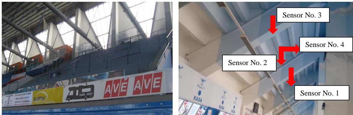
Fig. 1. The view on the observed grandstand sector, where the most active home fans are usually gathered (left) and the bottom view on the same sector with the location and orientation of the accelerometers used in the experiments (right).
