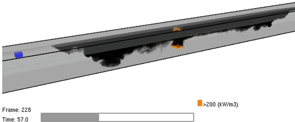
Fig. 2. 3D visualisation of smoke development [2].
