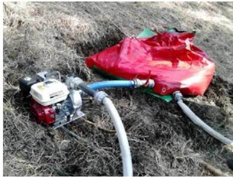
Fig. 1. The connecting of a pond with pump and hoses (photo: author)
