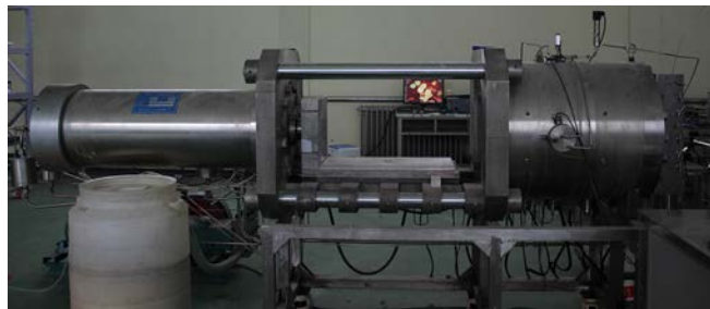
Fig. 1. RTM-1 large scale tri-axis hydraulic fracturing physical simulation apparatus.
