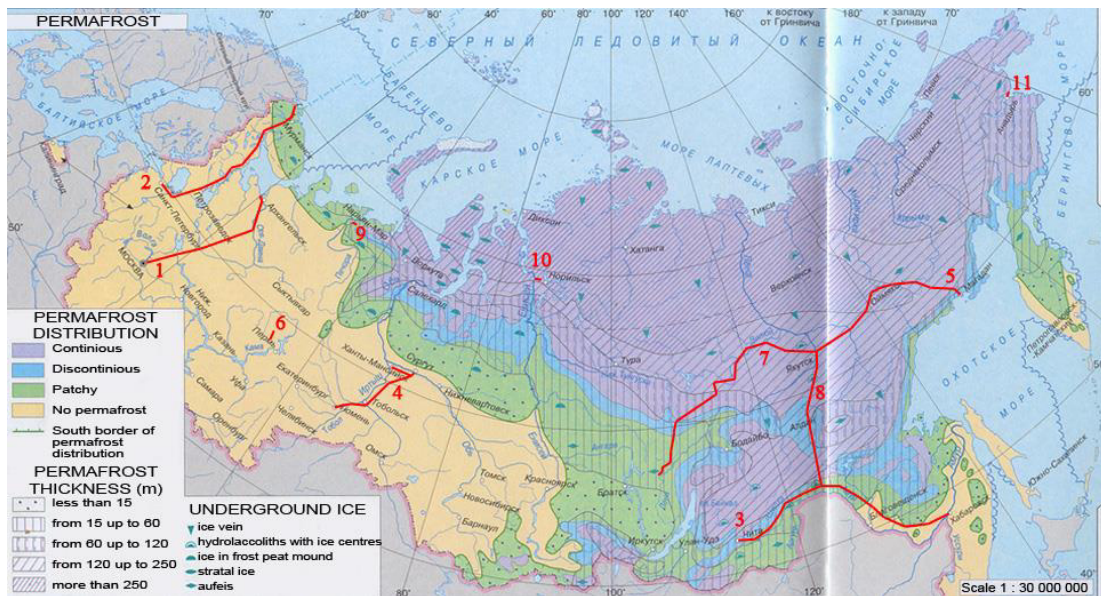
Fig. 1. Public Federal roads location on the map of territories with cryotic soils (Russian Federation): 1 – “Kholmogory” Moscow - Arkhangelsk (sections); 2 – “Kola” St. Petersburg- border with the Kingdom of Norway (sections); 3 – “Amur” Chita - Khabarovsk; 4 – Tyumen - Tobolsk - Khanty-Mansiysk; 5 – “Kolyma” Yakutsk – Magadan; 6 - Nytya – Kudymkar; 7 – “Vilyuy” Tulun – Yakutsk; 8 – “Lena” Never – Yakutsk; 9, 10, 11 – the access ways to the Naryan-Mar, Dudinka and Anadyr airports.
