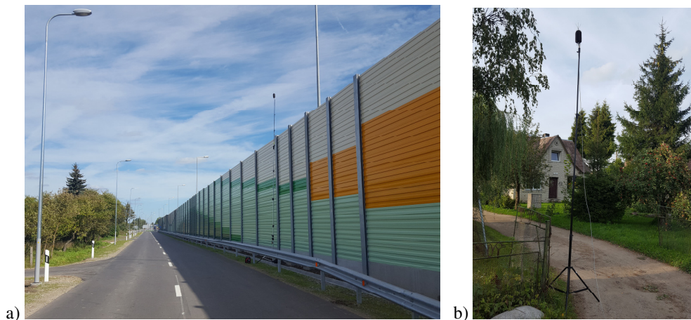
Fig. 1. Local connection road in the noise protected area and reference microphone point above the barrier (a); interested site point with 4 m height microphone (b).
